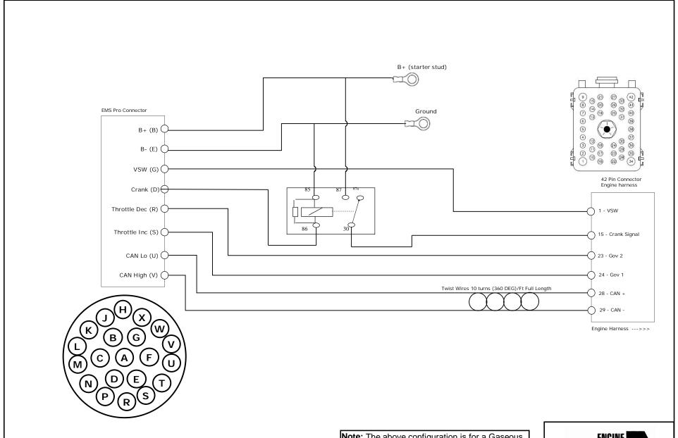
**Note:** The above configuration is for a Gaseous fueled engine. For Gasoline add the positive and negative to (Plns 5 and 18) to the Ford 42 pin connector. From those pins go directly to the fuel pump. Do not directly ground the fuel pump.
